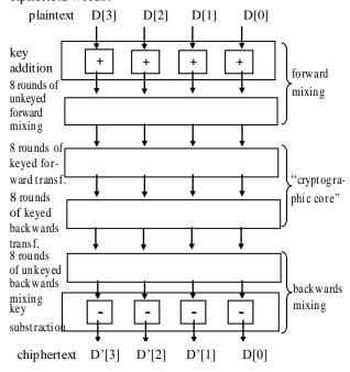
Figure 1. High-level structure of the chiper
