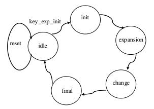
Figure 3. The state transition diagram for key expansion module
