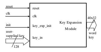
Figure 2. The detailed structure of key expansion module
