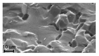
Fig. 4. SEM micrograph of BZT sintered in air for 4 h at 1550 °C—care zone.
