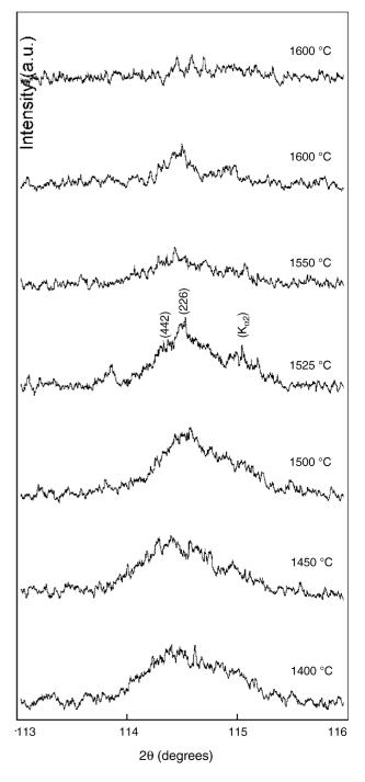
Fig. 2. The  $(2\,2\,6)$  and  $(4\,2\,2)$  reflection profiles of BZT ceramics vs. sintering temperature.
