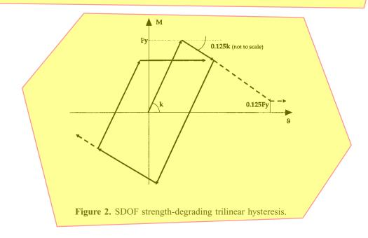
tility of approximately 2 and 6 under the target records. Viscous damping is always 5% of critical. For the most interesting moderate period case (T=1.5 sec case), a second trilinear backbone with a degrading strength branch (see Figure 2) is considered, again with two strength levels. Table 1 summarizes the SDOF structural configurations analyzed under both the target and the arbitrary groups of sets.
