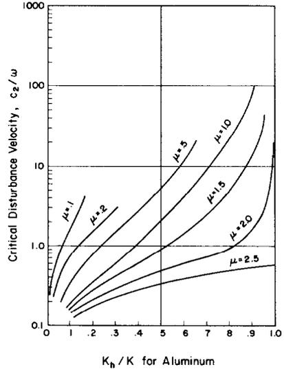
Fig. 2. Critical disturbance velocity in the less conductive body for a range of friction coefficients and for aluminum with hypothetical reduced conductivity sliding on aluminum.
