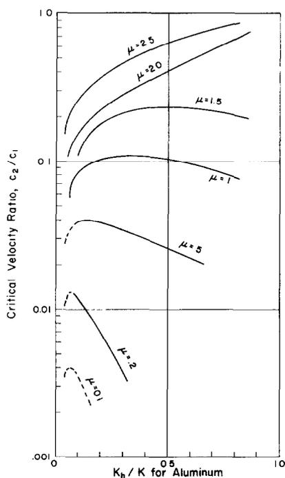
Fig. 4. Ratio of disturbance velocity in the insulator to disturbance velocity in the conductive body for aluminum sliding on aluminum with hypothetically reduced conductivity.
