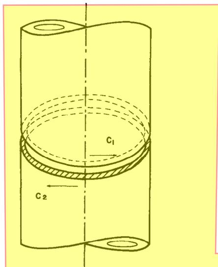
Fig. 1. Illustration of the geometry of thin tubes contacting end to end with sliding along the line of contact.
