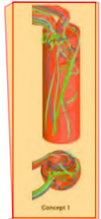
Figure 2: Particle tracking ribbon plots of the computed steady-state flow fields for two different port concepts
