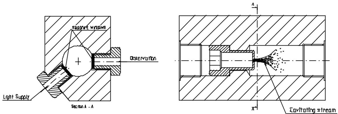
Figure 8. The arrangement of flow visualisation in the cavitating-jet apparatus.
