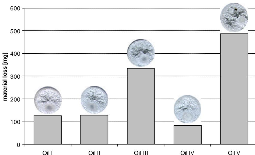
Figure 5. Material loss due to cavitation erosion with different oil types [Koivula et al. (1999<sup>a</sup>)].
