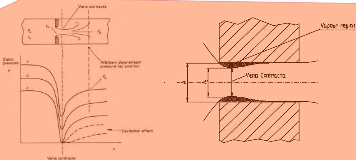
Figure 2. Pressure distribution at steady state flow in ideal orifice flow. At certain stage flow separates in orifice inlet corner and a vena contracta is formed.
