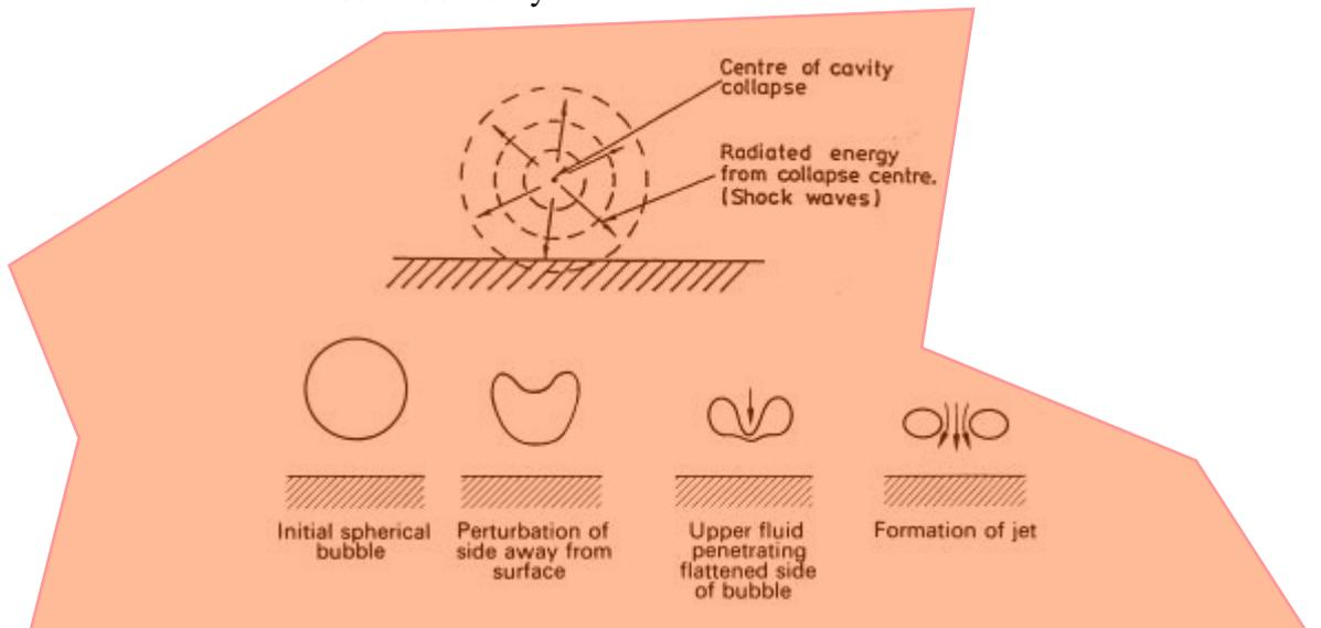
Figure 4. The shock-wave mechanism and micro-jet mechanism of cavitation erosion. [Lamb (1987), Knapp et al. (1970)]
