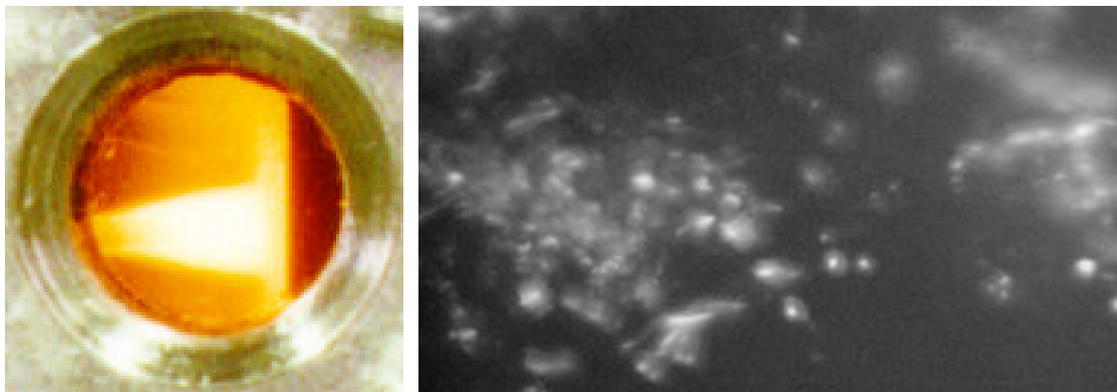
Figure 9. Photographs of cavitating oil flow. Left: halogen light and film-camera. Right: Close-up view with xenon-discharge light and CCD-camera.
