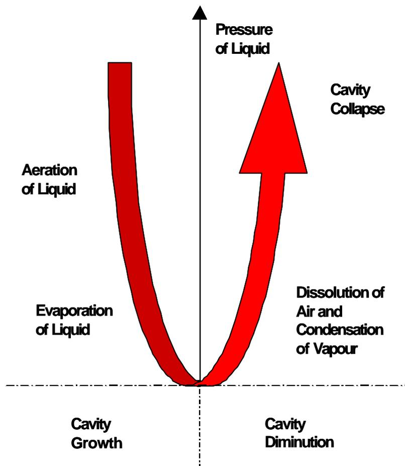
Figure 1. Cavitation process
