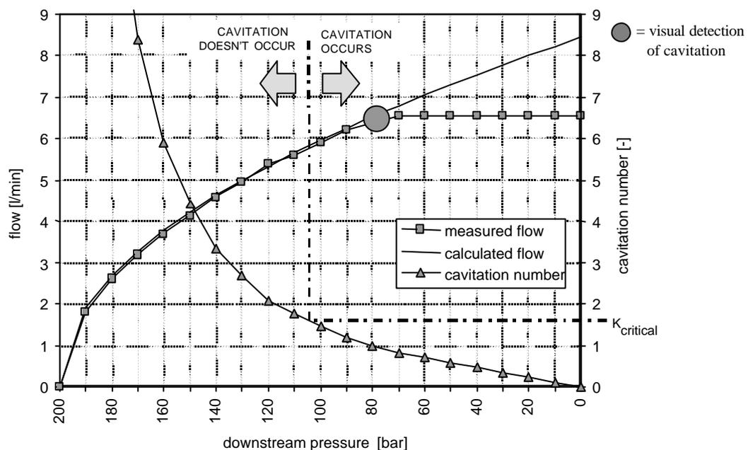
Figure 3. Comparison of measured and calculated flow rates through an orifice.
