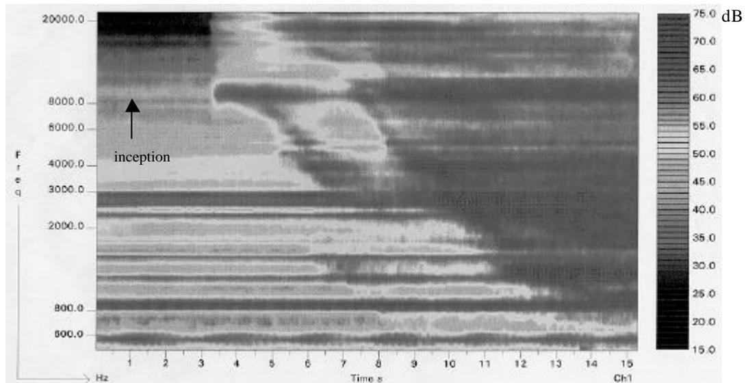
Figure 7. Frequency spectrum of acoustic pressure. Cavitation is developing when downstream pressure is decreased with time. [Koivula et al. (2000)]
