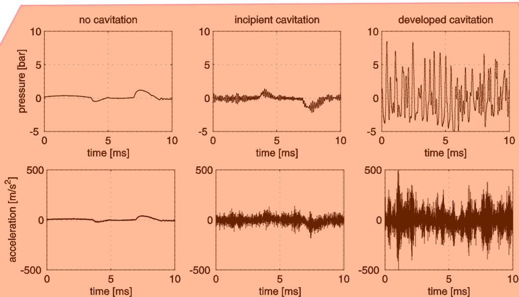
Figure 6. Pressure in downstream chamber and acceleration of the test block. Cavitation intensifies from left to right. [Koivula et al. (2000)]
