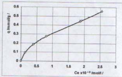
Fig.3. Ion-exchange isotherm of NRS on Amberlite IRA 402-Cl. Batch method: m/v=1 g/500 ml; stirring time, \tau = 2 h; t = 25 °C.
