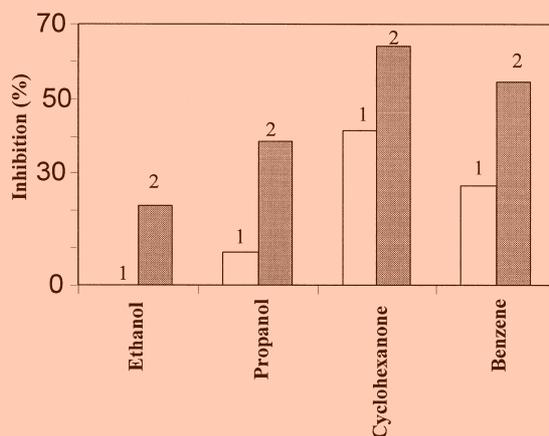
Fig. 3. Inhibition of acetylcholinesterase on the electrode surface after a 10-minute incubation in (1) 10% water–organic solvent mixture and (2) pure organic solvent.
