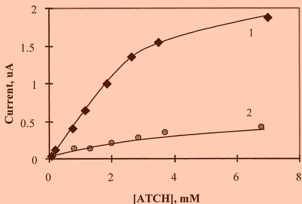
Fig. 2. Calibration plots for the ATCh in 0.1 M phosphate buffer (pH 7.5) containing 10% water–ethanol mixture, 0.1 M KCl, 0.01 mM  $MgCl_2$  and stirred at 300 rpm. Potential is 0.35 V versus Ag/AgCl; 20°C. 1) AChE-PB-PEI modified electrode; 2) AChE-modified electrode.
