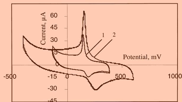
Fig. 1. Cyclic voltammograms of (1) PB and (2) PEI-PB modified graphite electrodes in 0.5 M KCl solution, 50  $\text{mV s}^{-1}$ , 300 rpm, 20°C.
