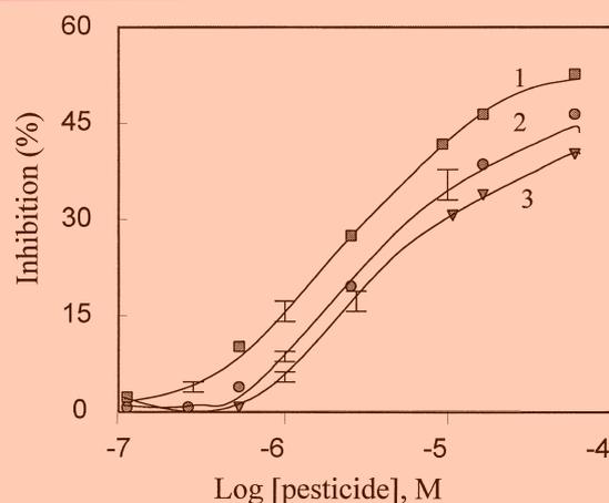
Fig. 4. Determination of pesticides with the AChE-PB-PEI modified electrode. Experimental conditions: 0.01 ml of pesticide in pure ethanol solvent was injected into electrochemical cell with 0.3 ml 0.1M phosphate buffer, pH 7.5, containing 0.1 M KCl, 0.01 mM  $MgCl_2$  and 0.1 mM ATCh at 300 rpm and at 20°C. (1) Dichlorvos; (2) Diazinon; (3) Fenthion. Error bars denote deviations for  $N = 5$ . Technique of measurement is the kinetic approach.
