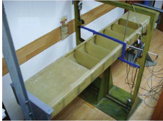
Figure 10: Ship hull model and torsion rig.
