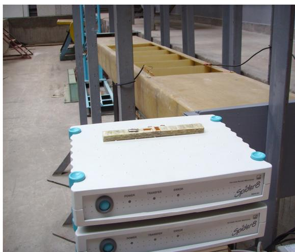
Fig. 11. Torsion rig for experiments.
