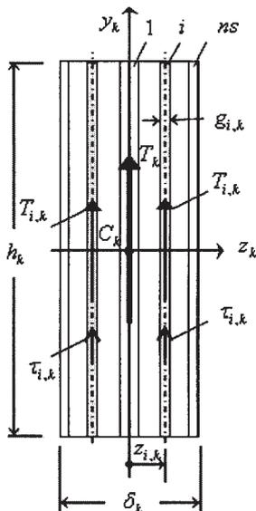
Fig. 6. Determination of equivalent shear stiffness
