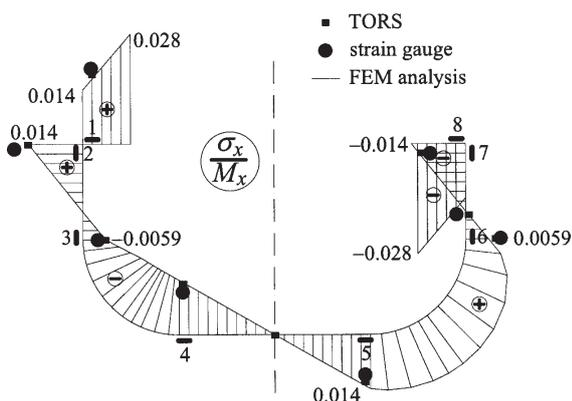
Fig. 13. Relative normal stress in the midship open section
