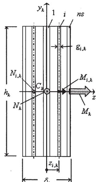
Fig. 5. Determination of equivalent bending stiffness
