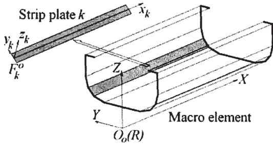
Fig. 1. Thin walled beam macro element
