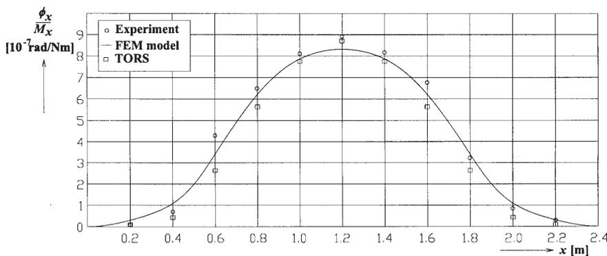
Fig. 12. Relative torsion angle along the ship model
