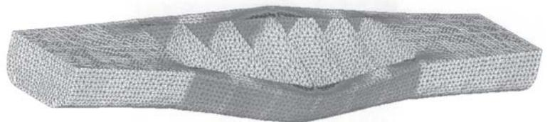
Fig.11. Ship model deformed due to torsion
