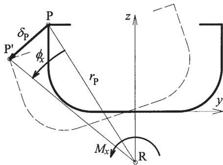
Fig. 8. Torsion angle calculus
