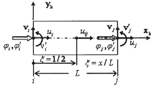
Fig. 3. Finite strip element
