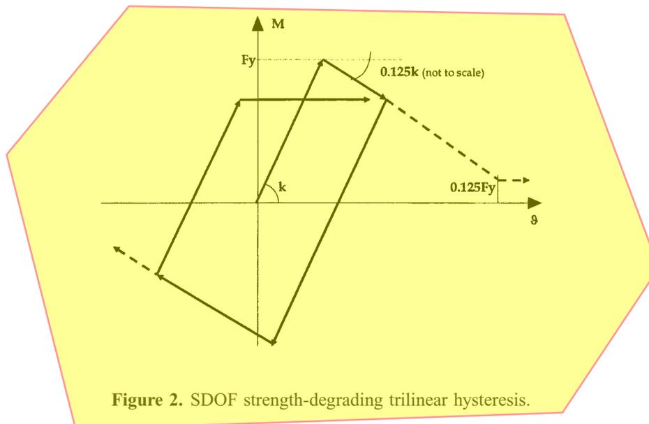
Figure 2. SDOF strength-degrading trilinear hysteresis.
