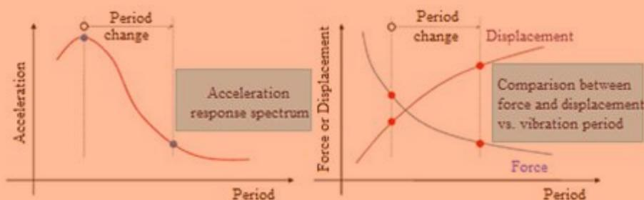
Fig. 1 – Theoretical principle of base isolation (Cruciat, 2013).
